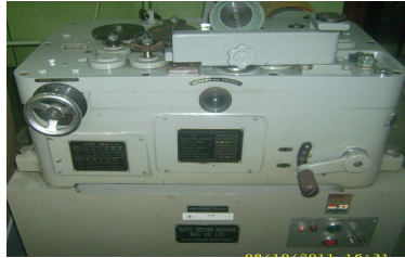
Gambar 3 Ogoshi High Speed Universal Wear Testing Machine (Type OAT-U) Gambar 4 Spesimen uji keausan
