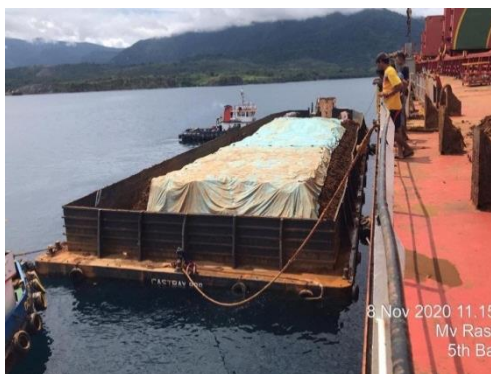
Gambar 11. Crew Tanpa APD saat Proses Barge Tender
